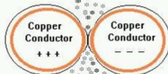
Electrons accelerate toward the conductors & bombard the insulated surfaces, eroding the protective layer like tiny sandblasters
